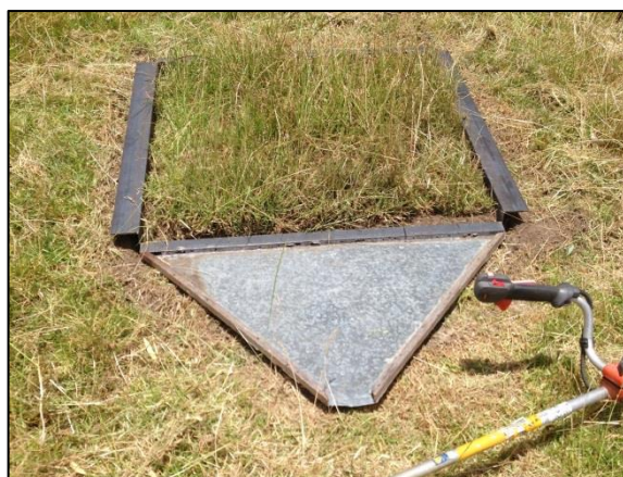
One-square metre field plot with run-off collection tray
